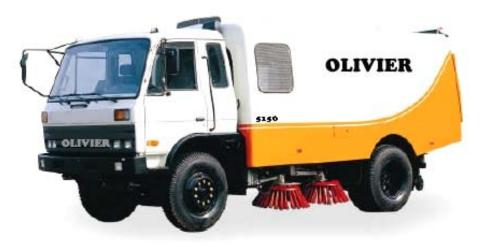
**Feature:** the new generation suction sweeping road sweeper is mainly used in sweeping the city road, bridge, square, airport, dock and so on. Original "four brooms in the Center-rear nozzle" overall structure arrangement, wide sweeping width, short front axle suspension, creative nozzle with international horizontal broom, greatly increasing the effect of cleaning.
