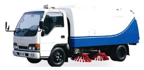
**Feature:** The new generation road sweeper made by Chinese Standard Company is mainly used in sweeping the city road, bridge, square, airport, dock and so on. Original" four brooms in the center-rear nozzle" overall structure arrangement, wide sweeping width, short front axle suspension, easy change the hose and adjust nozzle.
