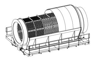
The secondary trommel falls on a hopper that guides the material on to the collection-up conveyor to the refining compost building, hereafter described.
